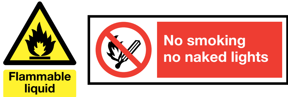
Figure 3 Example of warning and prohibition signs with supplementary text used at entry points to flammable liquid facilities
