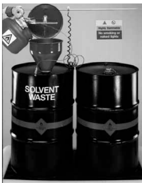
Figure 2 Example of system for waste solvent collection
